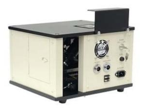
**International Patent** PCT: WO2018/056121 This machine is available to measure stress distribution of chemically tempered glass which is strengthened by ion-exchange from Li+ to Na+ using scattered light photoelasticity. In case of that the glass is strenghened by mixed liquid KNO3 and NaNO3, K+ layer should be measured by FSM-6000 and Na+ layer should be measured by SLP-2000. These data can be combined by special software.
